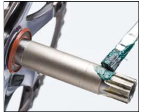
Figure 26. Greasing the axle
